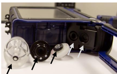
Fig. 57: Seal rings of condensation trap and condenser
