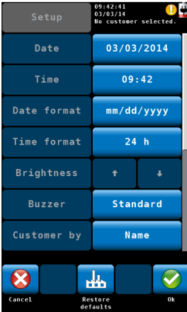
Fig. 52: Setup menu, the scroll bar shows that there are more parameters available.
