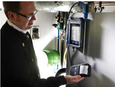
Fig. 32: Printing the readings of the Wöhler A 550 on the Thermoprinter Wöhler TD 100.
