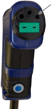
Fig. 48: Connectors at the probe handle. Guide bush marked by an arrow (only Wöhler A 550).
