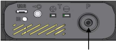
Fig. 47: Negative Pressure Connector at the bottom of the analyzer.
