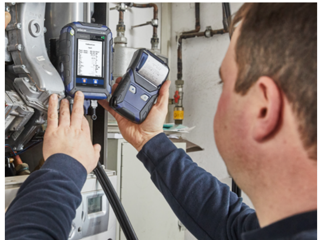
Interface to the printer Printout of the measured data on site.
